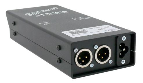
Rear side features the mains connector (so called mickey-mouse plug) as well as the two intercom connectors. The latter are standard 3 pin xlr male microphone connectors (Neutrik). A line termination circuit stabilizes the audio intercom signal. For those instances you should have no xlr female connector on hand, we have a simple solution: We supply a Neutrik gender changer (NC3FF) with the PS101S.
