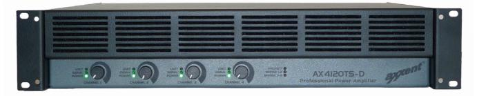
The professional audio amplifiers of the axxent TS series are optimised for use in fixed installations. The 4-channel model AX4120TS-D complements this series with an output power of 120 W/channel and 240 W mono bridged per pair. In addition to the analogue inputs, this model has a Dante digital input for easy networking. The switching power supply saves weight and increases efficiency and power balance.
