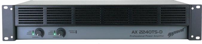
The professional audio amplifiers of the axxent TS series are optimised for use in fixed installations. The 2-channel model AX2240TS-D complements this series with an output power of 240 W/channel and 448 W mono bridged. In addition to the analogue inputs, this model has a Dante digital input for easy networking. The switching power supply saves weight and increases efficiency and power balance.
